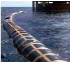
These are hoses for connecting tankers anchored offshore and onshore facilities and transporting crude oil. Since the hoses are installed in the special environment of the ocean, abundant experience and advanced technical capabilities are required for design that fulfills durability requirements in order to withstand severe storms such as typhoons. There are only a very few companies around the world capable of designing and manufacturing marine hoses.
