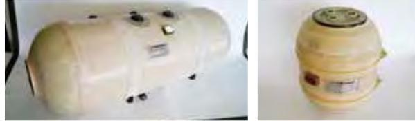
This is a drinking water tank for an aircraft. It has been manufactured by wrapping thread such as glass or carbon fiber impregnated with plastic such as epoxy above an inner liner that has been molded seamlessly, and it meets high resistance to pressure and acceleration while having a low weight. It has been manufactured with materials that are suitable for drinking water under standards such as the US FDA and NSF-61.
